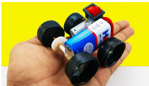
Figure 4.19: Simple car consisting of a battery glued to straws, a switch, a motor, a back and a front axle with wheels and two gears which connect the motor to the front axle. https://www.instructables.com/id/How-to-Make-MINI-Electric-CAR-DIY-at-HOME-Easy-Sim/
